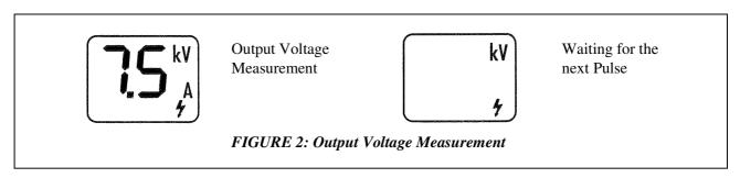
Your Smartfence Energizer features a low Output voltage Alarm (OA). If Output voltage drops below 3kV (factory default setting) and the Energizer, even at maximum Stored Energy, is unable to re-establish 3kV then the audible Output Alarm is activated. The Output Alarm can be either turned OFF, or set at 2kV, 3kV or 4kv consult your Gallagher Dealer or National Distributor if you wish to change the default setting. The symbol 'A' is displayed (Figure 2) when the Output Alarm is set.
