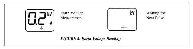
Your Smartfence Energizer features an Earth voltage Alarm (EA). This is an audible alarm which is activated when Earth Voltage goes above 500 volts (factory default setting). The Earth Alarm can be either turned OFF, or set at 300, 500 or 700 volts - consult your Gallagher Dealer or National Distributor if you wish to change the default setting. The symbol 'A' is displayed (Figure 6) when the Earth Alarm is set.
