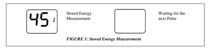
Stored Energy can therefore be used as a measure of fence condition. If, for example, a Smartfence MX5000 is showing a stored Energy reading of 30 Joules (or a Smartfence MX25000 is showing 12 Joules) your Energizer is well loaded but plenty of capacity remains to cope with a greater loading. However, if a Smartfence MX5000 is reading 40 Joules or greater (equally a Smartfence MX2500 is reading 20 Joules or greater) then the fence
