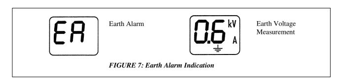
Note: The Earth Alarm indicates that the quality of the earth needs to be improved for optimum fence and "Remote" performances. Ideally the Earth reading is as low as practical.
